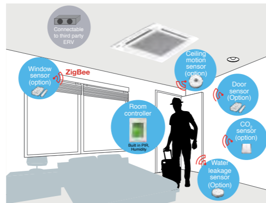
Batteries last for up to five years (10-year battery for CO 2 sensor) and are easy to install and replace.
